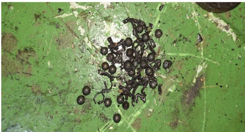
**Gambar 11. Patahan *Roller Ball Bearing* Pompa *Ballast***
