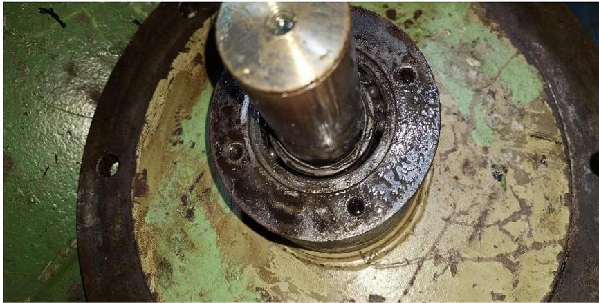
**Gambar 12. Roller Ball Bearing Pompa Ballast Rusak**
