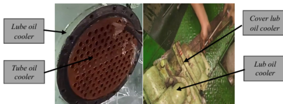
Gambar 10. Penggantian Packing Oil Cooler
