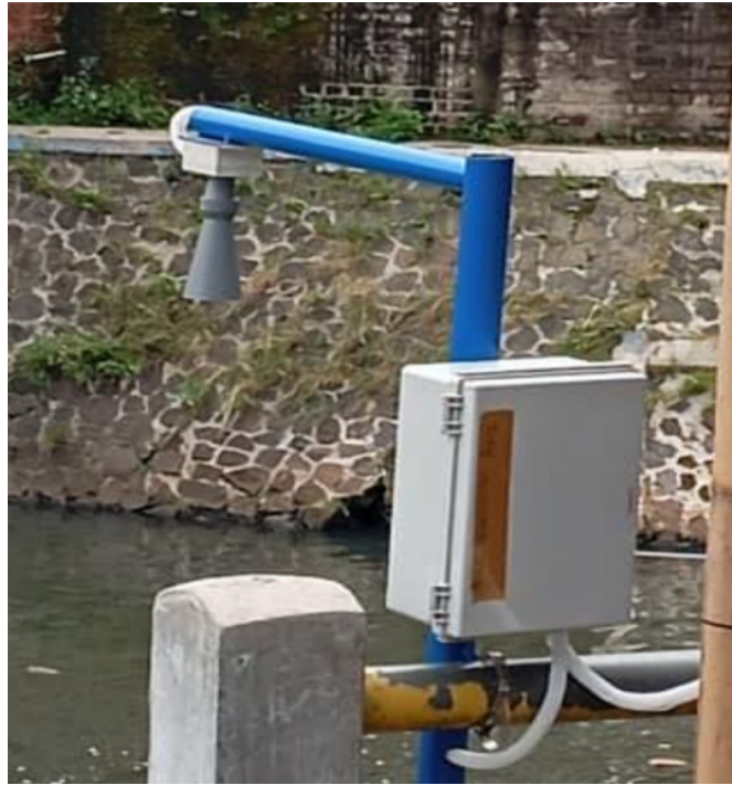
Figure 5. Sensor Measuring Water Level
