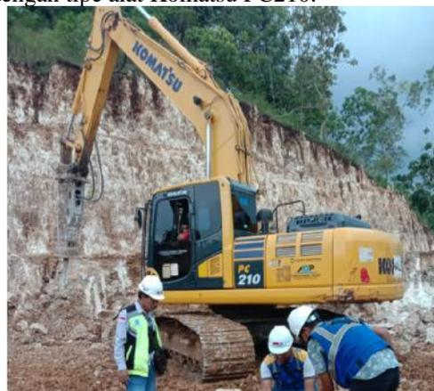
Gambar 1. *Rock Drill Breaker* (Komatsu PC210)
